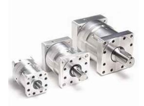
The LT Series is unique in that its zero backlash characteristic is maintained for life and high ratios of 50:1 to 200:1 are achieved in a single stage, thereby reducing length and weight as compared to traditional planetary designs which require multiple stages. The proprietary harmonic and cup designs allows for a high number of teeth to be engaged, giving the LT Series higher torque and inertial loading capacity, along with zero backlash, repeatability better than 10 arc-sec.
